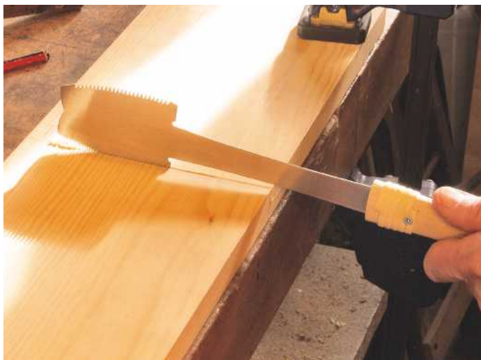
▲ Pic.6 Cutting a stopped housing with an azebiki
